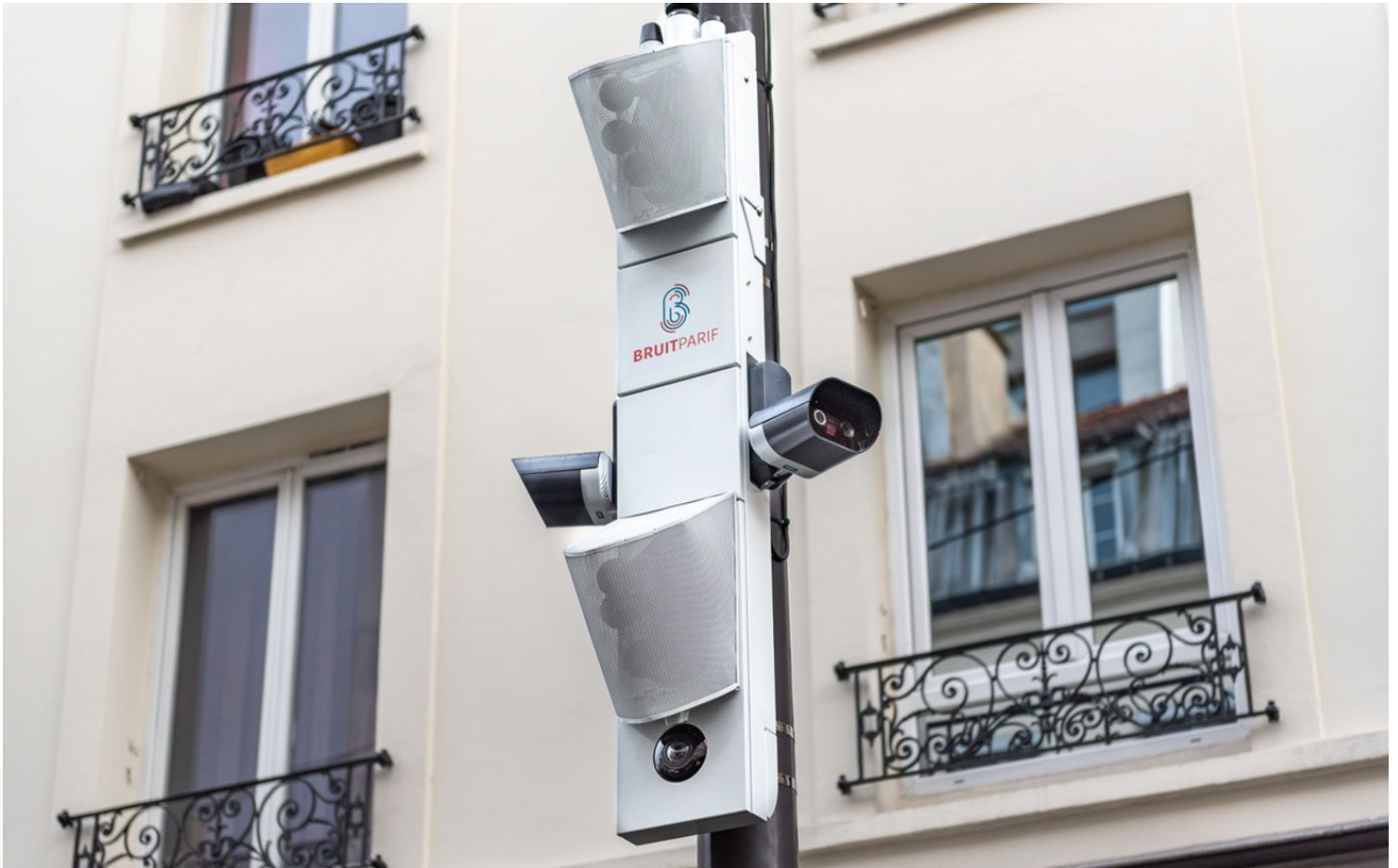
A sound radar device in Paris combines microphones and cameras to detect noise offenders. Photographer: Clement Dorval/Ville de Paris
