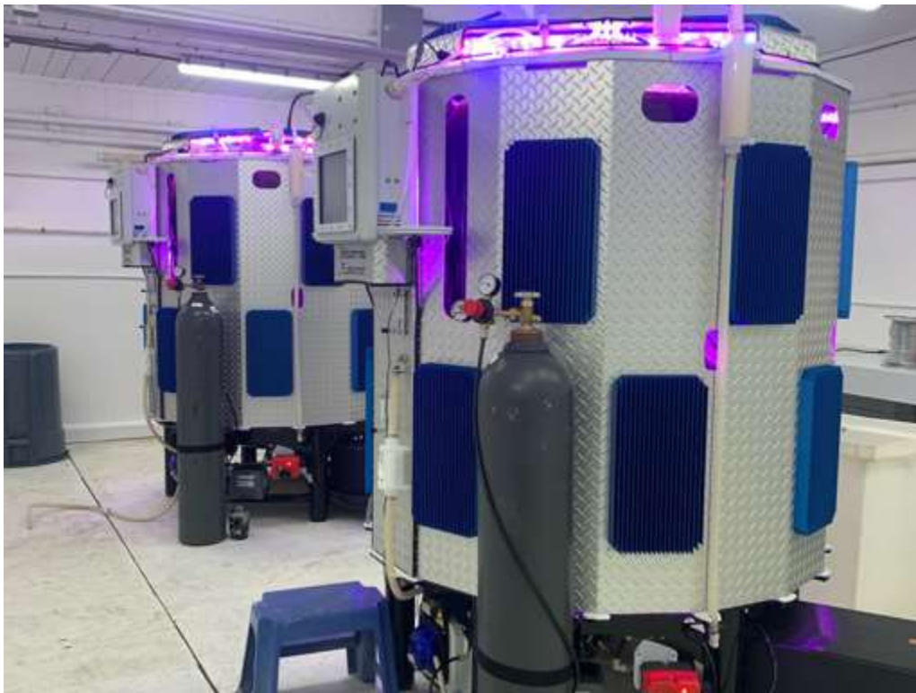
Fig.5. Photobioreactors (PBR) used to culture microalgae. Note these self-contained units are highly biosecure and minimize bacterial and protozoan contamination of the algae culture.
