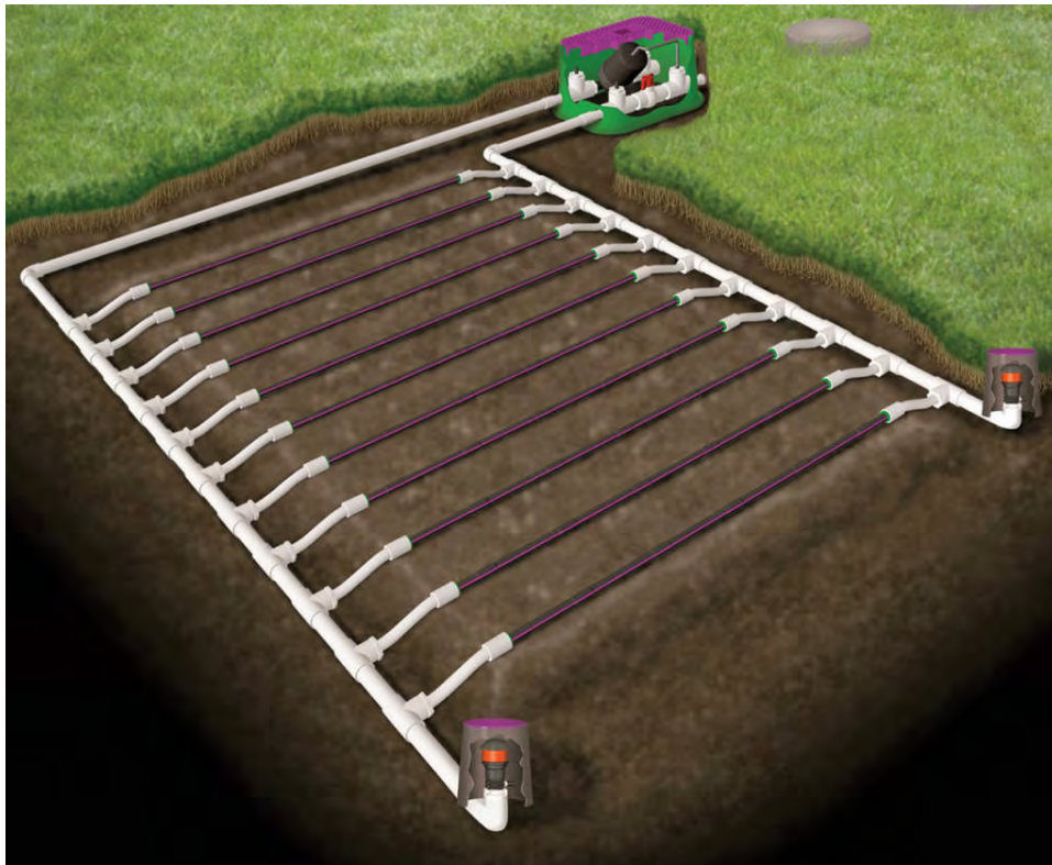
Figure 3.23 Drip Irrigation System
