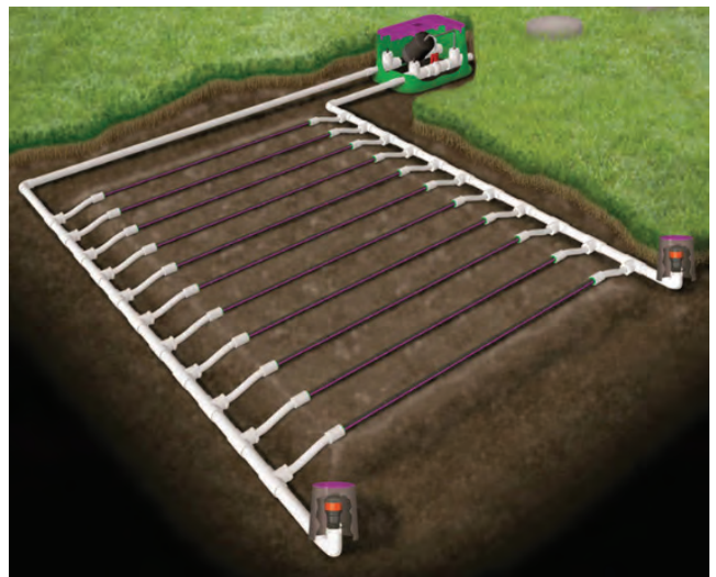
High-Pressure Drip Disposal System.
