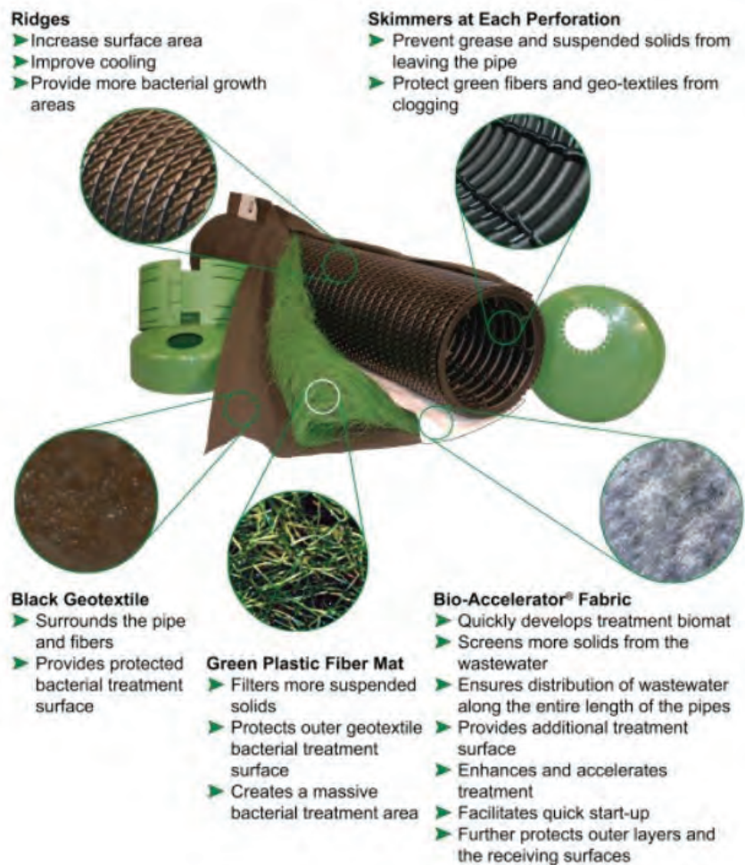
FIGURE 5. Presby Advanced Enviro-Septic® Treatment System. (Presby Environmental, 2018) Presby systems can be used in higher priority areas where nitrogen removal is required.
