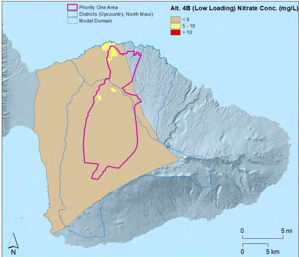
Figure AP5-5c. Nitrate Concentrations of Alternative 4B_LO: Cesspools Upgrade to Septic Tank to Seepage Pit with lower loading (1 persons/BR and 70 gal/person)
