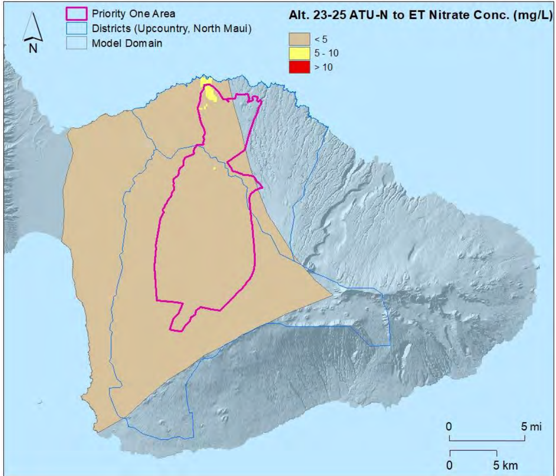
Figure AP5-21. Nitrate Concentrations of Alternatives 23A-25A: Sewer Pukalani and Cesspool Upgrades to Aerobic Treatment Unit-Nitrification to Evapotranspiration (smallest area >5 mg/L in alternatives 1-18) Elsewhere, as possible
