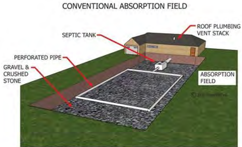
Figure 3.18 Absorption Bed Disposal System
