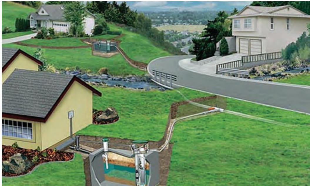
Liquid-Only Pressure Sewer System (Orengo Systems, Inc.).
