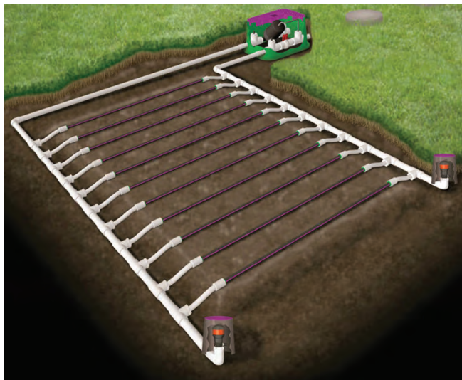
Drip Irrigation System.
