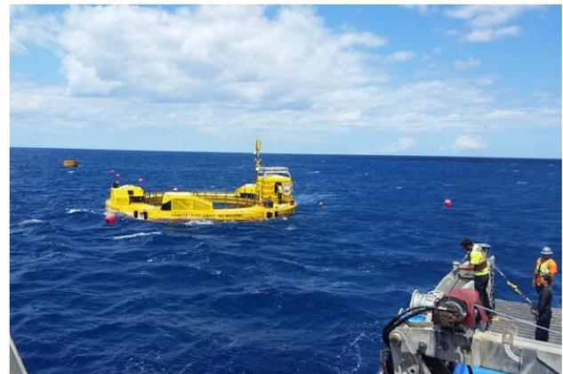
*February to August 2018:* HNEI led second deployment of Azura, with modifications designed to improve power performance, including enlarging the float and adding a heave plate at the base.
