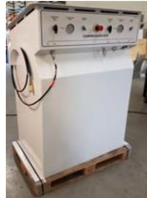
Figure 8: MTA Boost Compressor Fueling Post.
