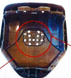
Emblem Improperly attached by melting with heat
