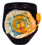
Genuine OEM inflators are precisely secured and carefully fitted over a metal plate to ensure that the inflator remains in its proper position in the event of a collision. Counterfeit inflators are often very loosely attached presenting a serious safety risk to motorists if the inflator were to deploy.
