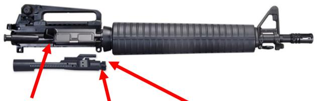
"Firearm receiver" means the part of a firearm that provides no using for the firearm's internal component, including a hammer, bolt, breechblock, action, or firing mechanism.
