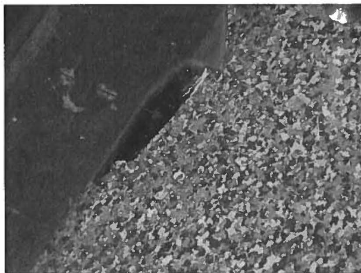
Sample no: 305-A5. Game Room-Lounge Area. Green-brown w/ speckles, 9" X 9" vinyl floor tile w/ black mastic. ACM 4% Chrysotile (floor tile) ACM <1% Chrysotile (mastic)
