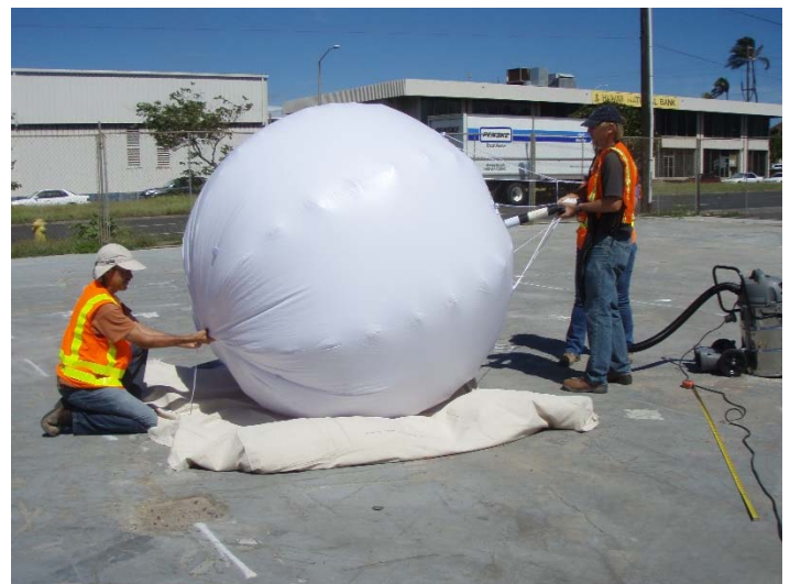
Innovative Approach – DOH and Contractors Collect Large Volume Vapor Samples at the Former Al Phillips Site.
