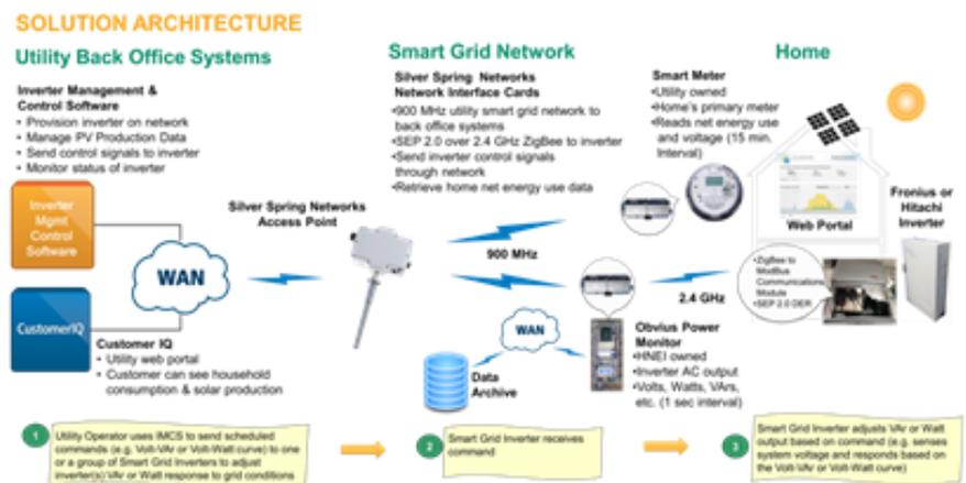
Figure 1. Project technology and solution architecture.
