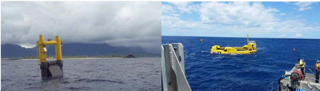
*Figure 6: Azura and Lifesaver wave energy converters deployed off of Marine Corps Base Hawai'i.*
