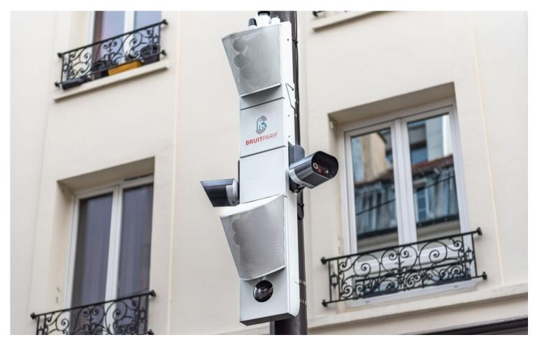
A sound radar device in Paris combines microphones and cameras to detect noise offenders. *Photographer: Clement Dorval/Ville de Paris*
