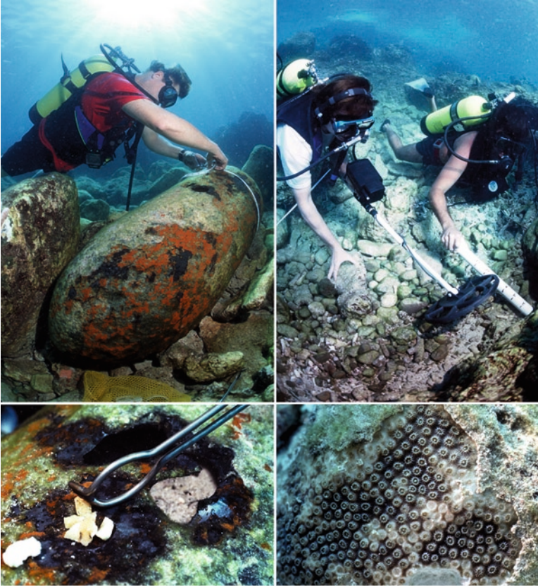
Fig. 4 ( Upper left ) Underwater unexploded ordnance (UWUXO) in high concentrations litters the seafloor in many areas around the world. Photograph shows a 2,000 lb General Purpose air-dropped bomb located at Site 3 (Fig. 1 [bottom]) just south of Roca Alcatraz within the US Naval bombing range, Isla de Vieques, P.R. This ordnance had several corrosion holes located in its mid-section exposing the contents of the bomb to the surrounding seawater. (Photograph by Dr. James W. Porter) ( Upper right ) Bomb craters pock mark coral reefs on the seaward side of Bahia Salina del Sur, Isla de Vieques, P.R. All craters investigated in the magnetometer survey were perfectly symmetrical holes, approximately 14 m in diameter and 1.5 m deep, such as this typical crater 50 m south of Roca Alcatraz (18° 07' 21.60" N; 065° 18' 03.50" W). (Photograph by Dr. James W. Porter) ( Lower left ) High explosives from within the cavities of a corroding bomb on the Vieques coral reef spill and leach out onto the surrounding reef. The granular material from these unexploded munitions was analyzed for TNT, Semtex, C-4, and other high explosive compounds. (Photograph by Dr. James W. Porter) ( Lower right ) Diseased colony of the mountainous star coral ( Montastraea faveolata ) in physical contact with a leaking bomb. Samples of this colony detected the presence of exceptionally high concentrations of explosive compounds. (Photograph by Dr. James W. Porter)
