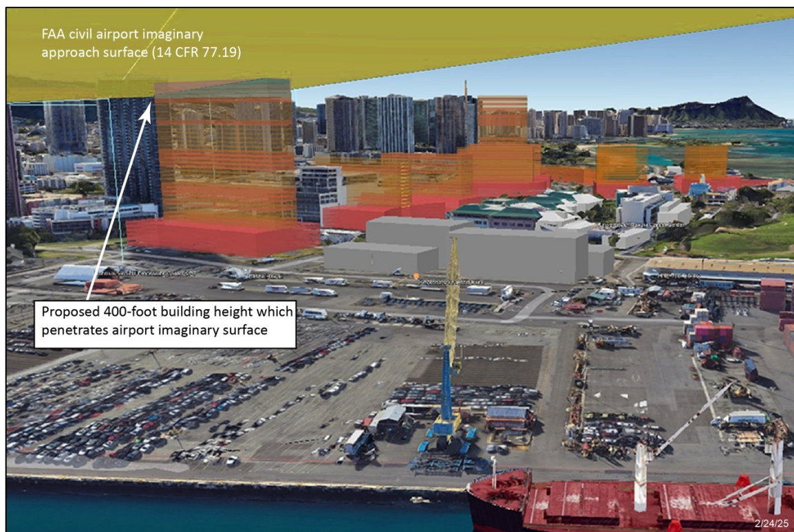
Figure 9: A view looking Diamond Head showing how one of the proposed 400-foot building sites in Kaka’ako Makai would penetrate the FAA civil airport imaginary surface from below, as pursuant to 14 CFR Part 77.
